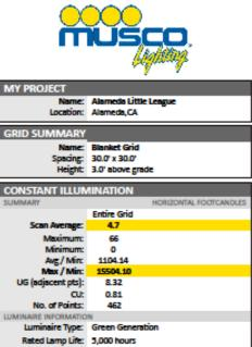
LUMINARE INFORMATION Luminaire Type: Green Generation Rated Lamp Life: 5,000 hours Design Lumens: 134,000 Ave Lamp Tilt Factor: 1.000 No. of Luminaires: 18 Avg KW: 28.15 (30.6 max)
