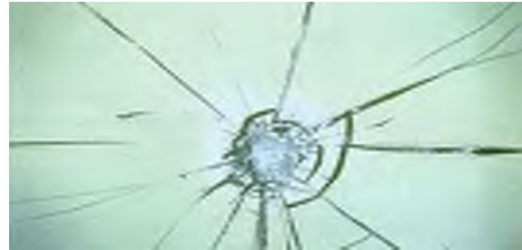
Laminated glass breaking pattern
