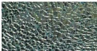
Tempered glass breaking pattern
