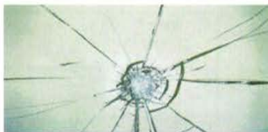
Laminated glass breaking pattern
